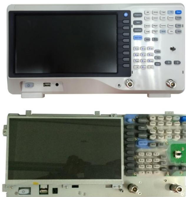
Figure 4-2 Removing the front panel
